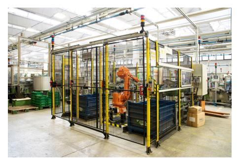
Figure 1.1: Industrial robot kept in a cage to prevent injuries from humans.
