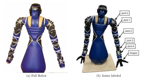
Figure 2.3: The *King Louie* soft robot from the BYU RAD Lab used with permission of the RAD lab
