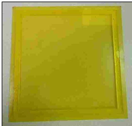
Figure 7: Fiberglass Mold Surface - Acrylic Boundaries
