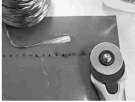
Figure 3: Set-up to Cut NCCF
