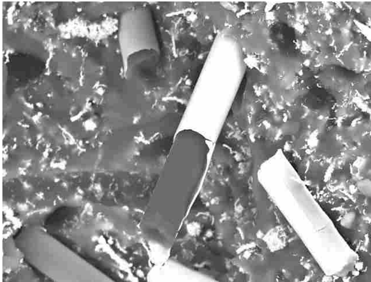
Figure 2: SEM EBSD Image of NCCF within Nanocomposite 3kX
