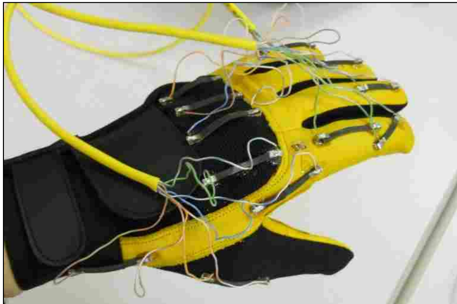
Figure 13: Prototype Glove with HDSGs and Connections
