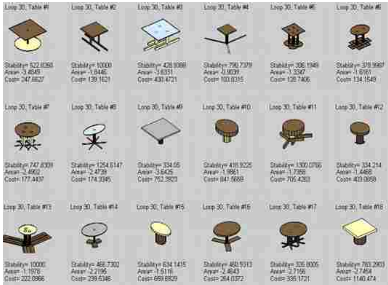
Figure 6.5: Table designs automatically formed consisting of new combinations of table features.
