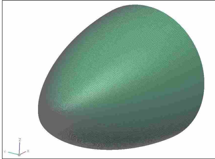
Figure 4-38: Example Rocket Fairing Structural Mesh (HAACK)
