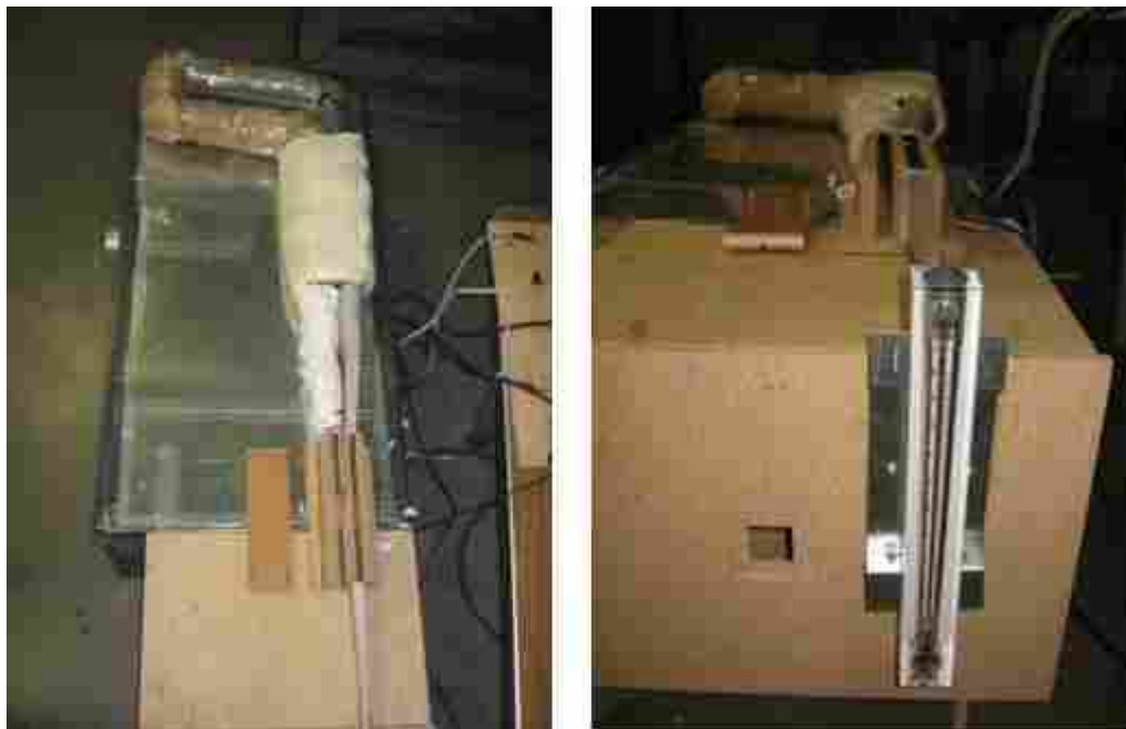
Figure 6-2: Photographs of Test Station. Left: View from above of the flow circuit. Right: Front view. Air passes up through the rotameter, which measures volumetric flow, and then enters a specially constructed box. The box contains two separate flow paths and holds a thermoelectric device and a heat sink exposed to each stream.
