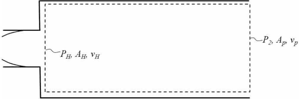
Figure 9: Control volume for a sudden contraction area when the flow reattaches within the baffle plate
