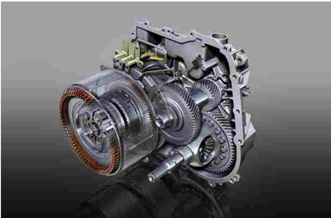
Figure 5.5: Chevrolet Volt Transmission [9]
