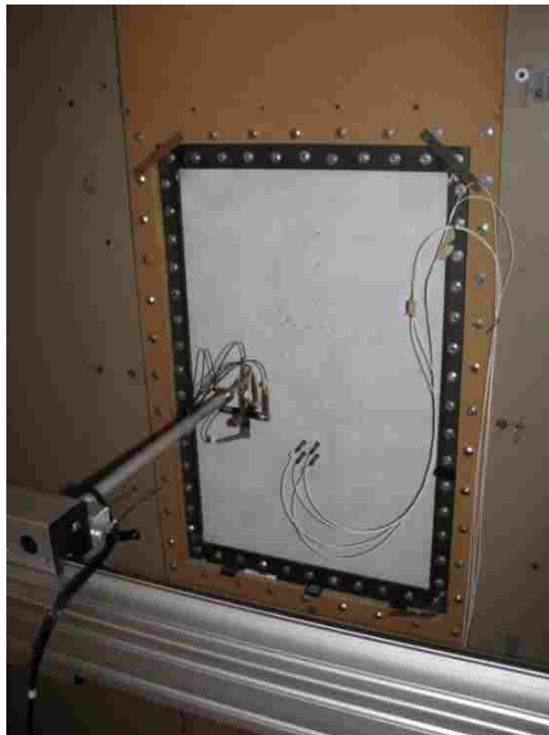
Figure 3-9: The experimental setup showing the scanning system in front of a clamped rectangular plate mounted inside a reverberation chamber.
