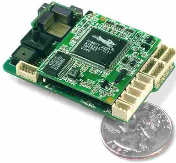
(a) Procerus Technologies Kestrel Autopilot
