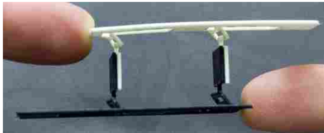
Figure 3.11: Actuated two-layer parallel-guiding MLEM (only actuates into open position)
