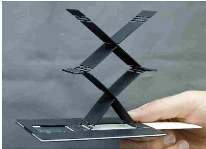
Figure 3.20: Nuremberg scissor MLEM repeated to show increased deflection in z-direction
