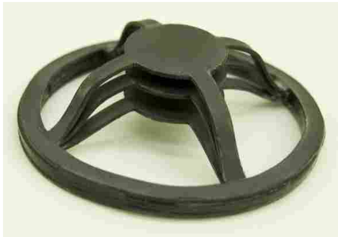
Figure A.4: Three-layer contact-aided MLEM
