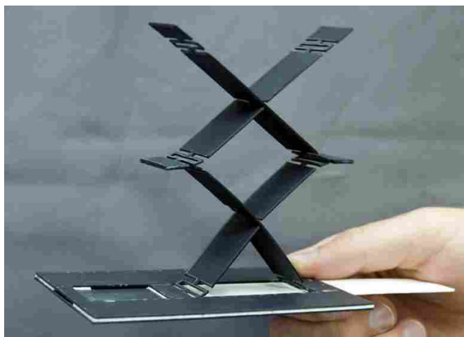
Figure A.12: Nuremberg scissor MLEM repeated
