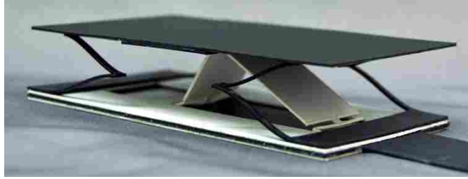
Figure 3.19: MLEM crank-slider pushes up on platform to separate layers
