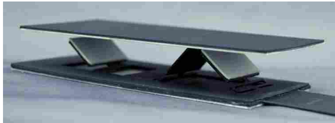
Figure 3.18: MLEM crank-slider attached to parallel-guiding mechanism to separate layers
