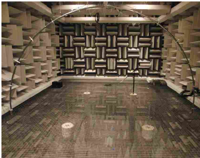
Figure 2-8: Picture of the 13 microphone measurement array in the anechoic chamber
