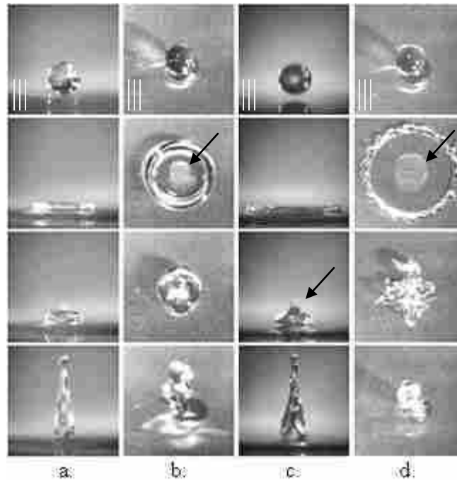
Figure 3-11: Images of droplets of the water/glycerine mixture impinging upon a coated structured surface (Cases 7-8) at We \approx 50 from a) the transverse view and b) the top view and We \approx 250 from c) the transverse view and d) the top view. Frames show, from top to bottom, the droplet at impact, at maximum spread, as a vertical jet is being issued, and as it is rebounding from the surface.
