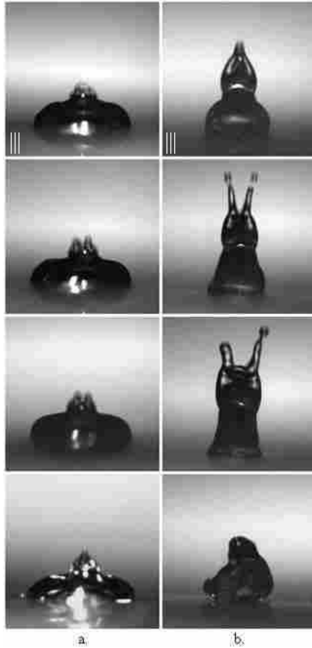
Figure 3-12: Images of the two-pronged jet phenomenon taken on a) a patterned uncoated surface (Case 3) and b) a patterned coated surface (Case 8). Values of We shown are, from top to bottom, a) 220, 250, 290, and 330; b) 195, 205, 250, and 270. All images were taken about 9 ms after impact. The top image of each set is at a value of We just before the onset of the two-pronged jets. The next two images of each set picture examples of two-pronged jets, and the final image of each set is at a value of We where the two-pronged jets are no longer observed.
