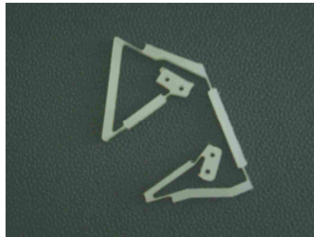
Figure 2.15: A prototype spring designed to follow a circular input path.
