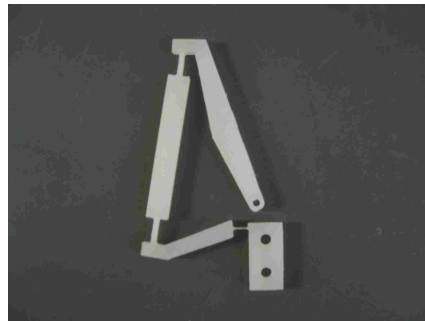
Figure 2.22: Prototype spring designed to approximate a zero-free-length spring.
