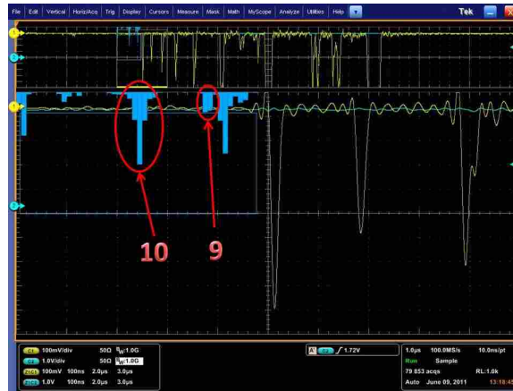
Figure 2.9 Zoomed-in oscilloscope histogram showing peaks from \text{Ar}^{9+} and \text{Ar}^{10+} inside the interaction chamber (28 mJ pulse energy).
