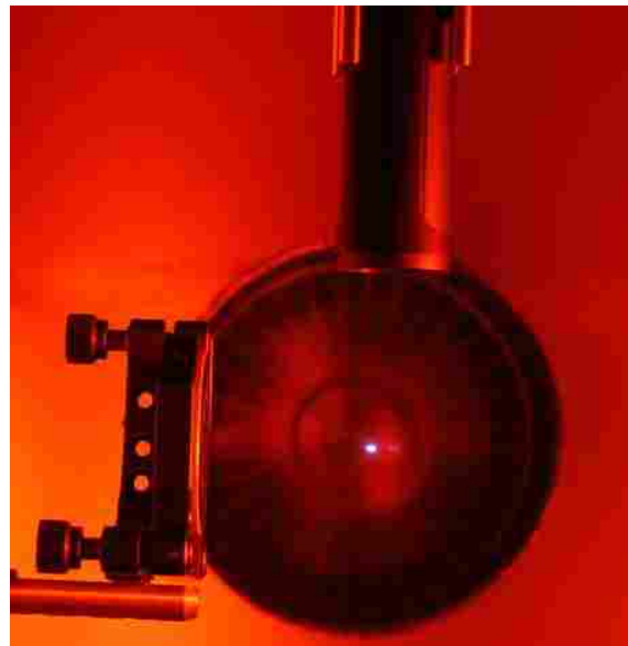
(b) Ionization at the laser focus
