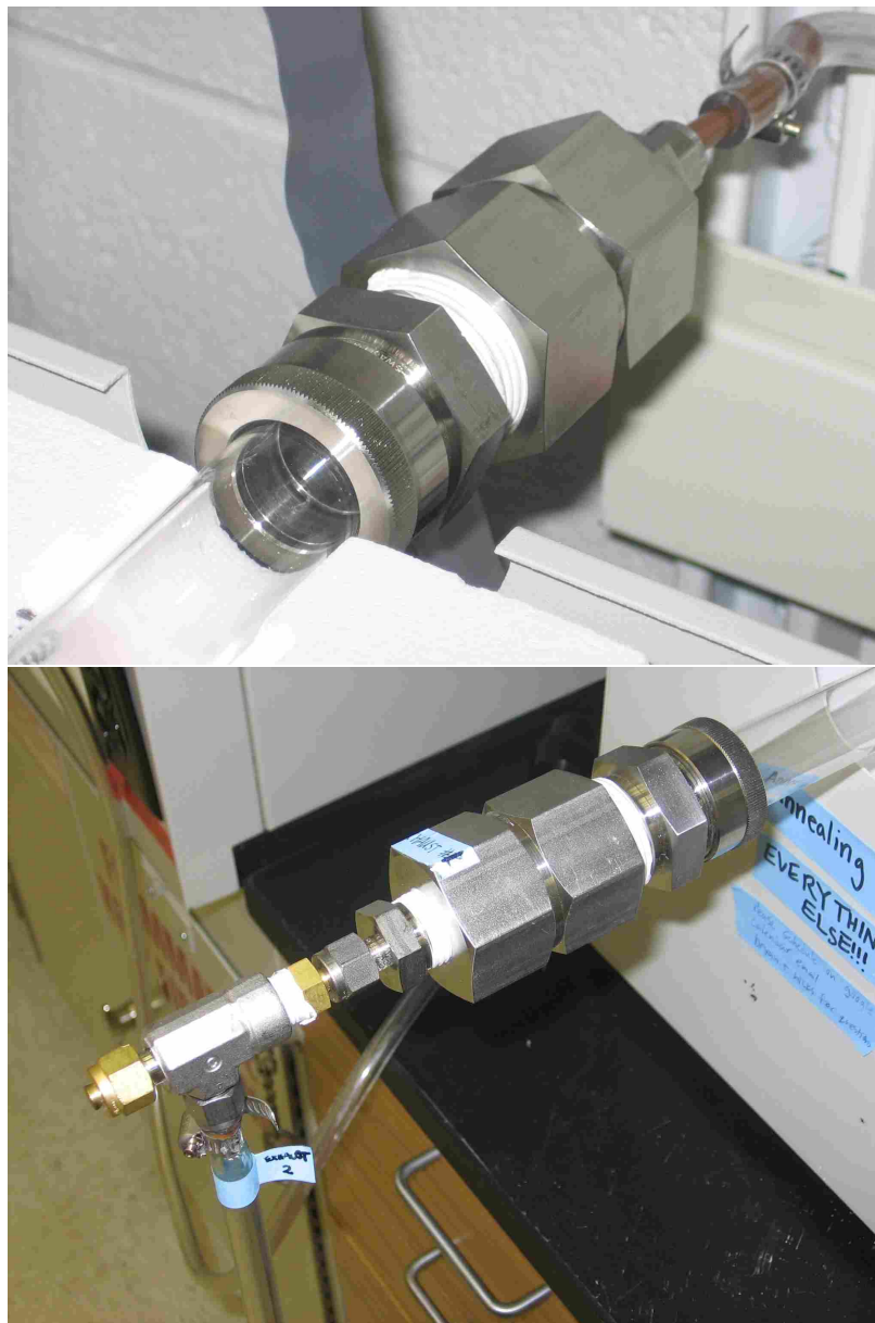
Figure 2.5 Both inlet and outlet to the quartz tube are fitted with a rubber “O”-ring to form an air-tight seal. Further, the outlet was outfitted with a “T” joint to allow a guiding rod to move the sample into and out of the “hot-zone.” (Here, the “T” joint is plugged as it is not being used)
