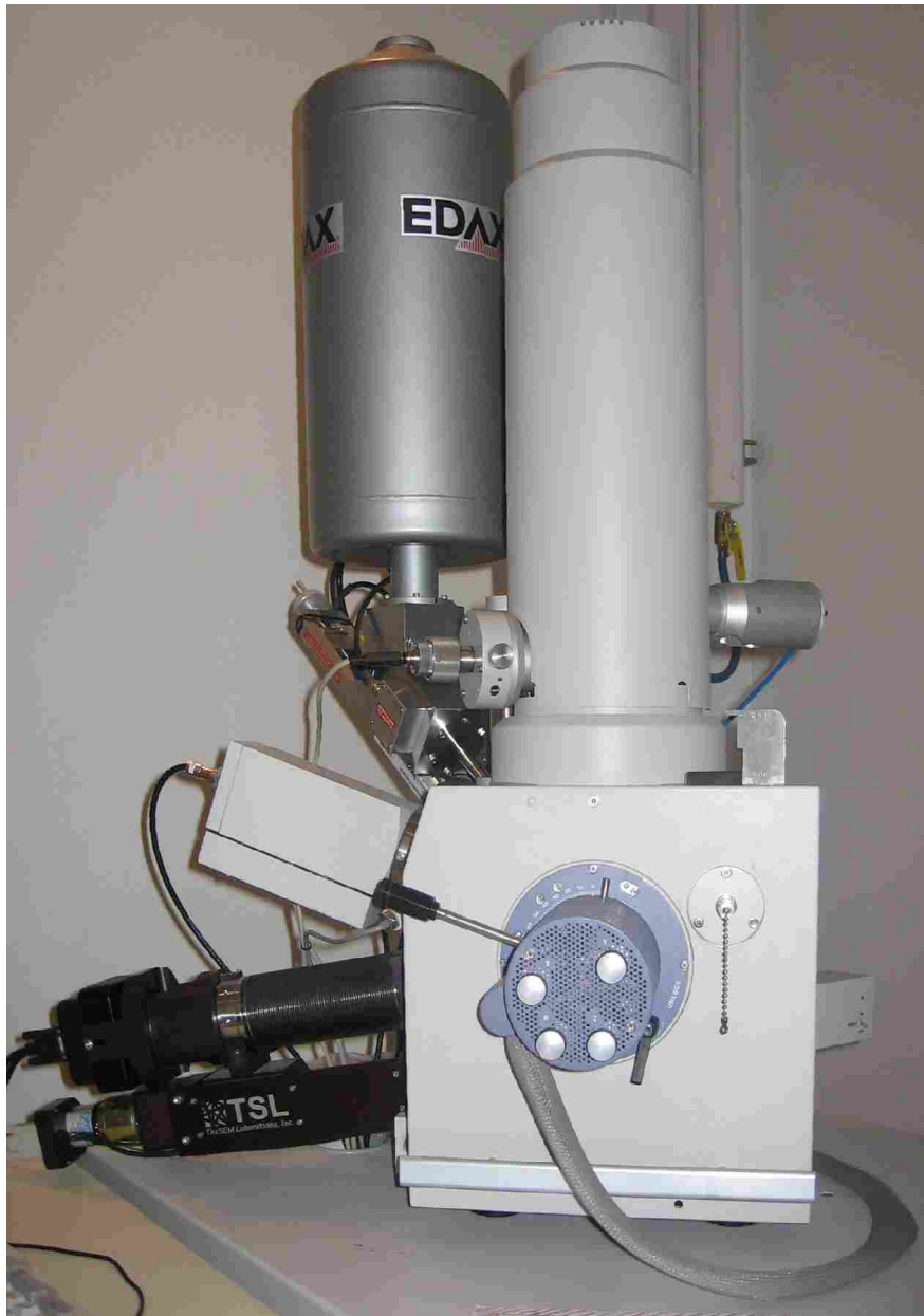
Figure 2.7 Phillips XL30 Scanning Electron Microscope. Shown in the picture are also the SE, the XEDS, and the EBSD detectors
