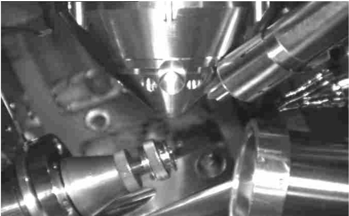
Figure 2.10 Interior of the Phillips XL30 SEM set for a tilted-view. The normal to the sample is 70° away from the beam. These conditions are necessary to perform an OIM scan. The EBSD detector has been inserted into the SEM.
