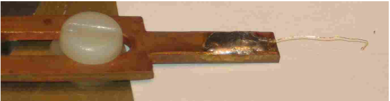
Figure C.4 Picture of a characteristic gold probe used for electrical measurements. The wire itself is used to provide a “springy” contact of the ball to the film.
