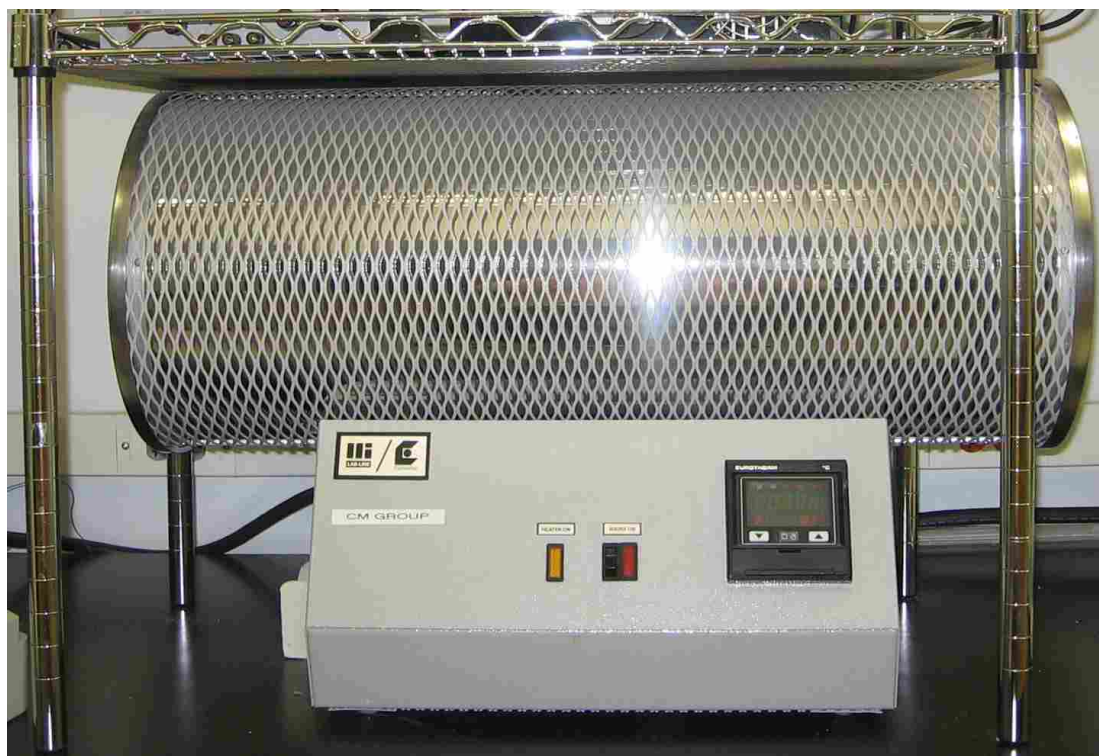
Figure 2.2 Furnace used for the anneals done in air.
