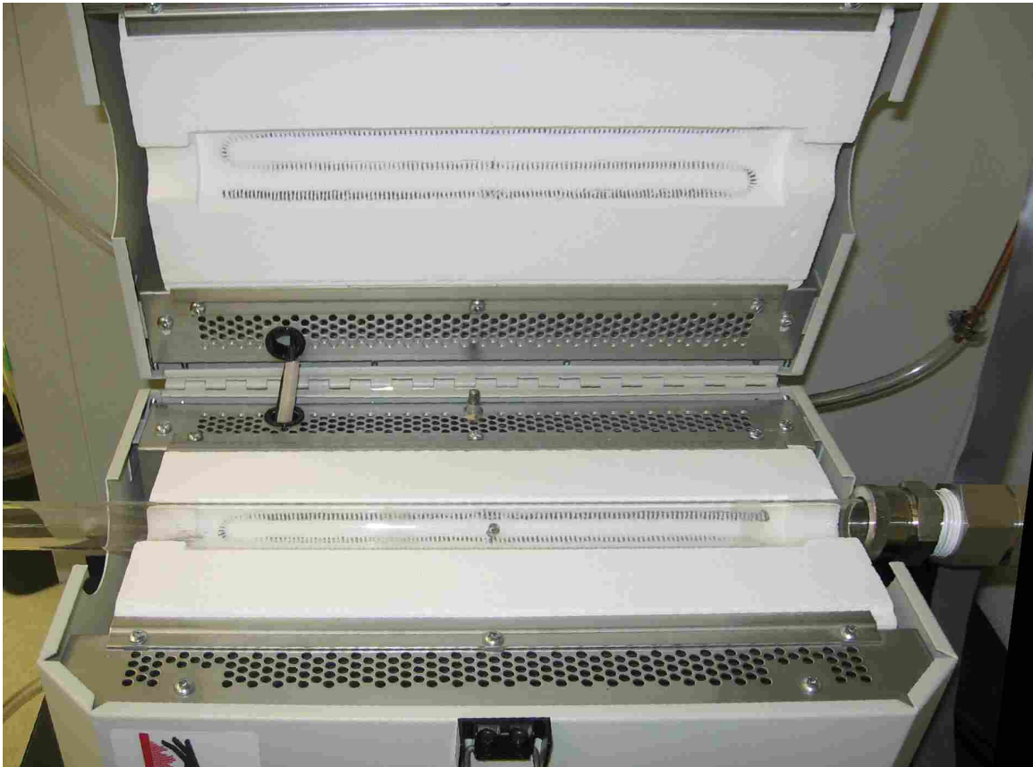
Figure 2.4 Furnace used to perform the argon anneals. The ability to open the furnace allows for easy placement of the sample close to the thermocouple (located in the middle).
