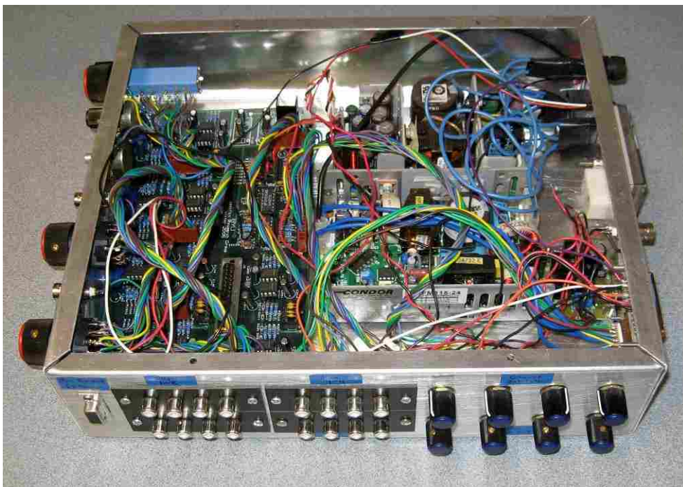
Figure 4.3 “Silver Box”- module containing variable filters and gains used to condition the inputs and outputs independently for the control system
