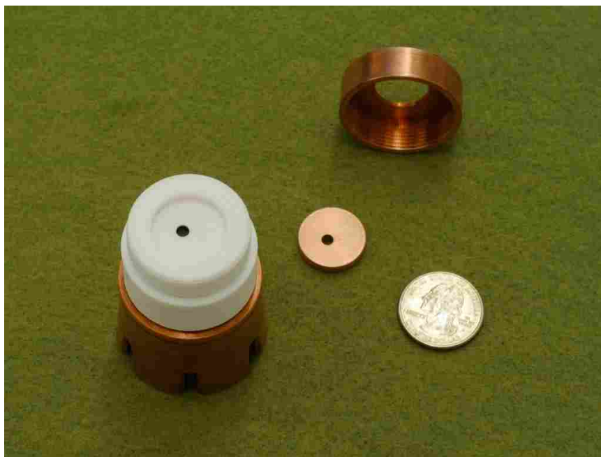
Figure E.2 The target and macor mask are placed onto the cathode base.
