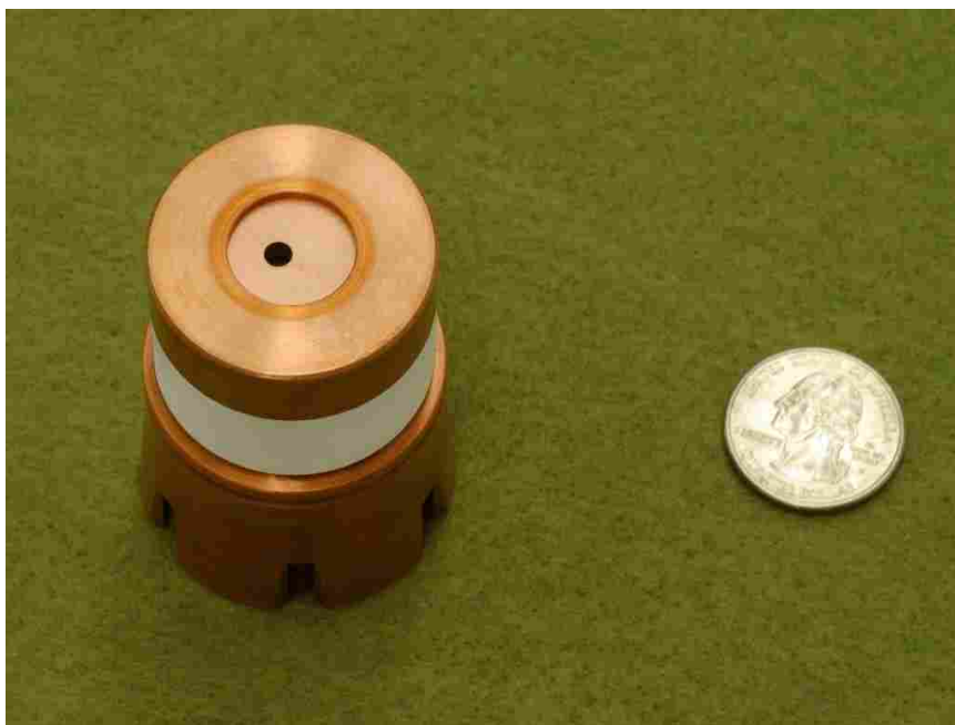
Figure E.4 The trigger disk is placed into the locking ring, aligned with the macor mask.
