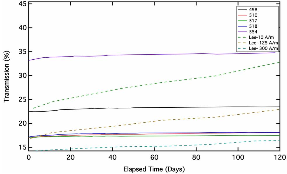
**Figure 2.4** Optical transmission of 5 different write layers were measured over 120 days at room temperature, shown in the solid lines. Optical transmission of bare tellurium films from Lee and Geiss is shown in the dashed lines for comparison.
