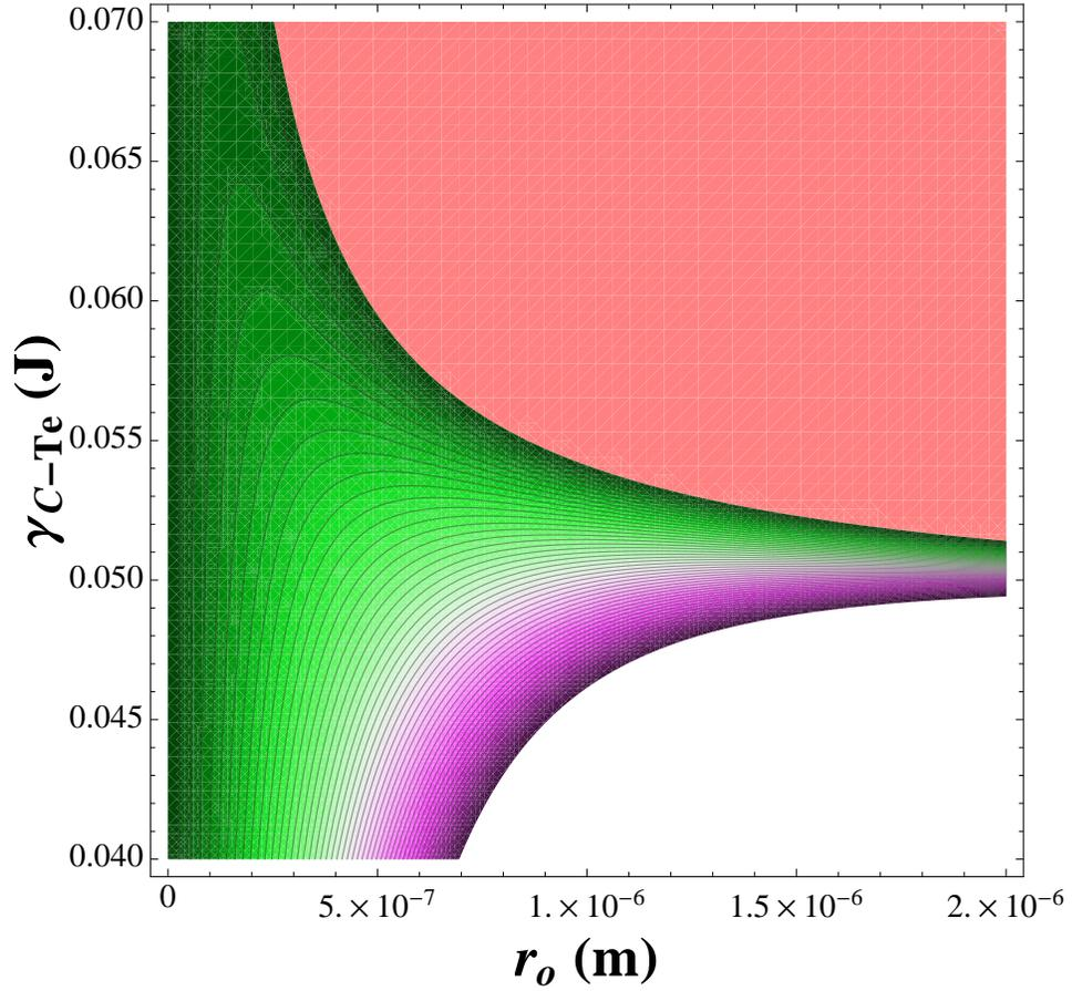
**Figure 1.3** The difference in surface energy before and after making a hole in the tellurium layer as a function of hole radius,  $r_o$ , and carbon-tellurium interface energy,  $\gamma_{C-Te}$ . The pink region is where  $\Delta E \leq 0$ , the white region is where  $\Delta E \geq 5 \times 10^{-14}$ .
