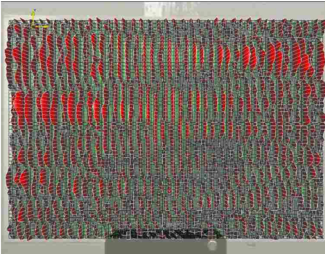
FIG. C.3. Scanning laser vibrometer measurement of the entire large plate.
