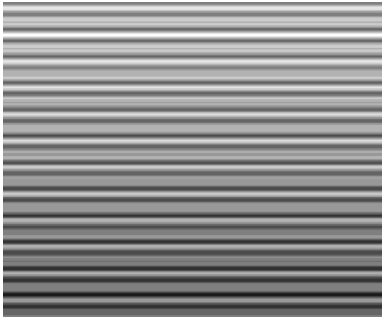
Figure 2.3 Typical background image created using the rtextimage program in IRAF. Each pixel in a given row corresponds to the midpoint value of that row found using the gstatistics program. The image is then used with the imarith routine in IRAF to subtract it from the image and remove the background.
