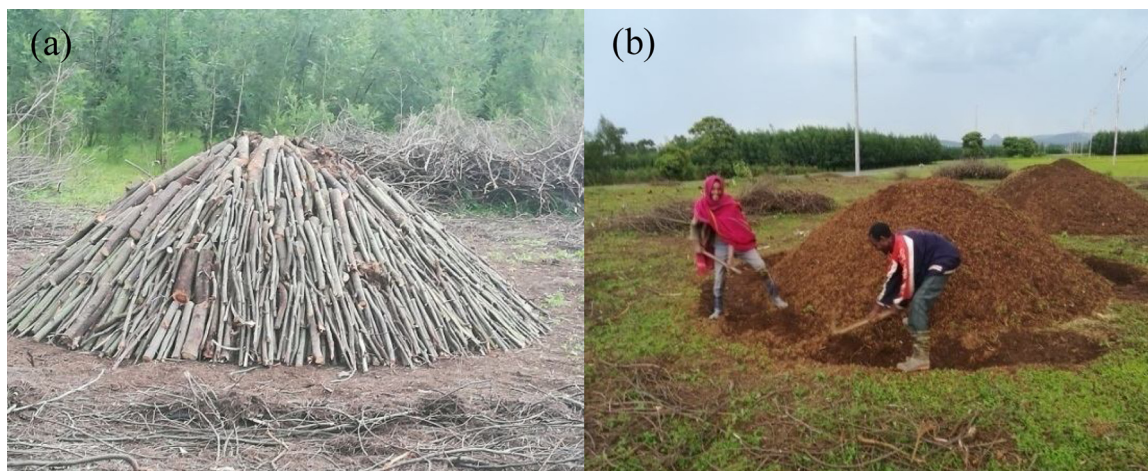
Fig. 2. Charcoal production (a) cut wood of acacia stacked for charcoaling (b) charcoal burners' preparing an earth mound kiln.
