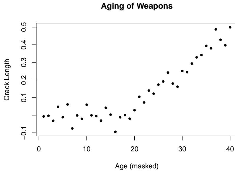
Figure 5.1: Masked crack length data from radiographs of weapons
