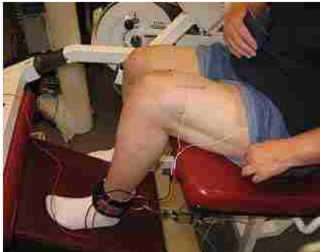
FIGURE 1. Quadriceps strength and activation testing. Strain gauge is attached to seat frame and to subject's ankle at 90^\circ to leg. Knee flexed to 75^\circ . Two electrodes were placed over the vastus medialis and proximal rectus femoris of the quadriceps.
