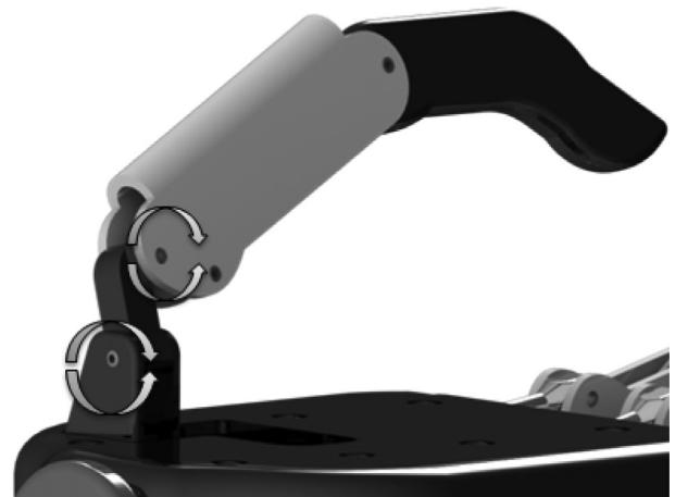
Fig. 2. The thumb architecture.
