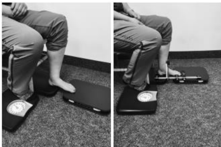
Figure 3. Arch height index measurement setup.
