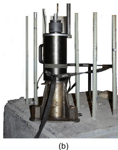
Fig. 2. Pull test arrangement. (a) A sketch and (b) the test arrangement.
